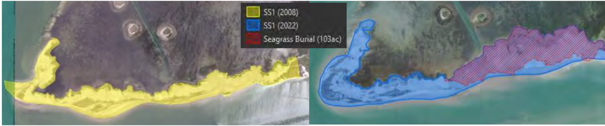
Figure 1: Historical and Recent Aerial Imagery Demonstrating Significant Erosion and Deposition of SS1, resulting in approximately 103ac seagrass burial.
